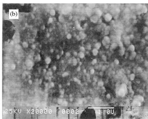
Fig. 3. SEM micrographs of gels from tetramethoxysilane solutions. The porous network was prepared at different concentrations of TMOS: (a) 20% (v/v) and (b) 10% (v/v).
